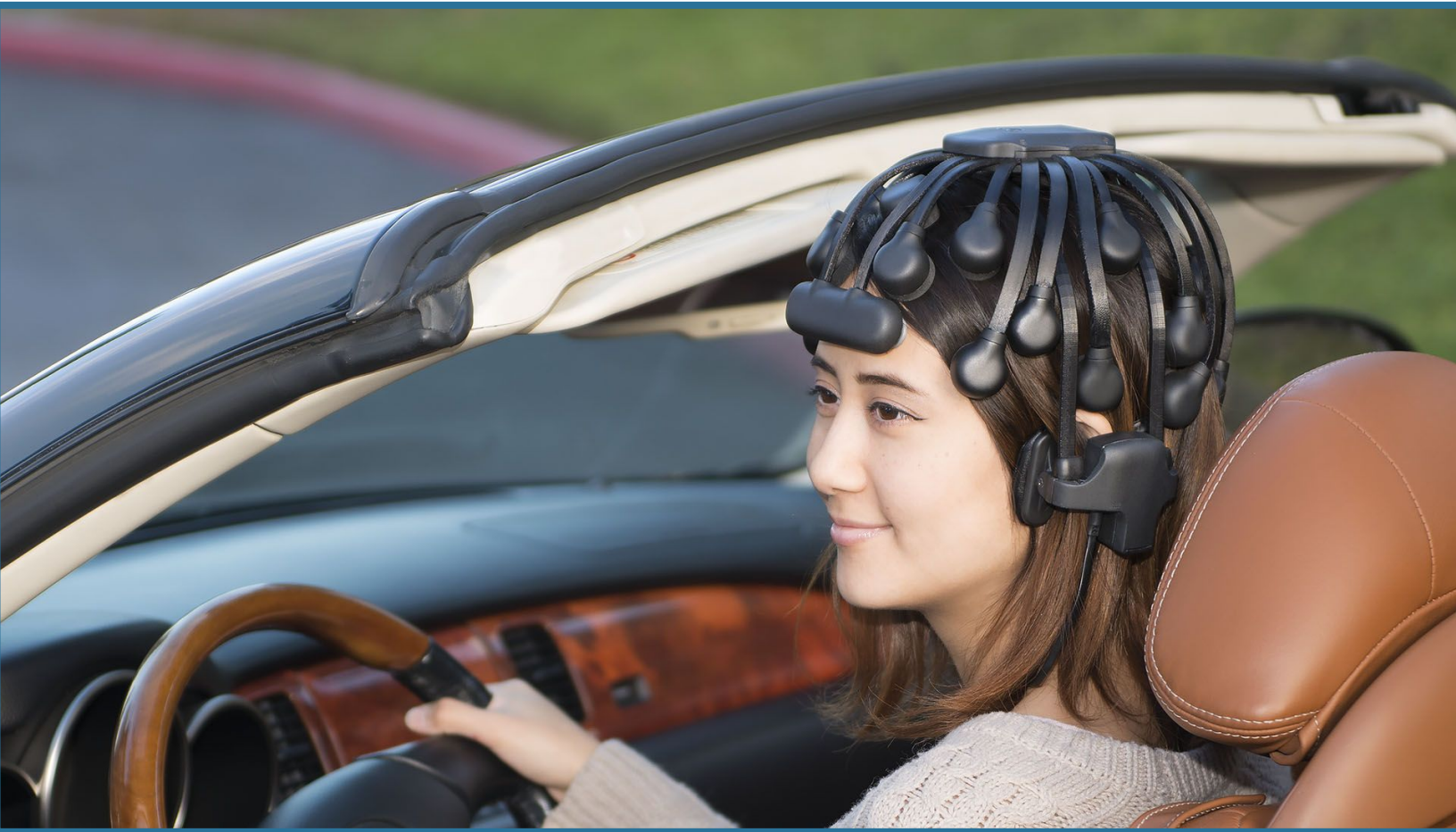
Quick-30: a wireless, dry EEG headset developed by Cognionics
